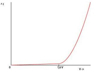
We detected the knee voltage by observing the LED, as from a certain value it started emitting light. The knee voltage is around 1,6 V.
