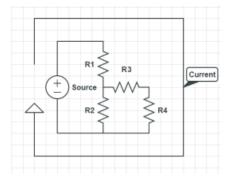
Write out the KVL for all closed loops of the circuit shown in Figure 6.2.
