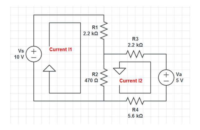
Image: Current I1 and Current I2 symbolize the current in this circuit, were in Current I1 is Loop 1 and Current I2 is Loop 2.
